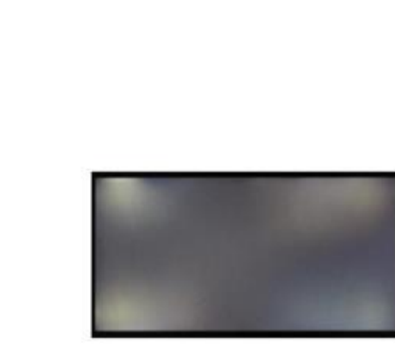
Fig.3 Lack of Softness LCD MURA caused by Stress at Lamination, and/or from the warpage of the cover plate.
